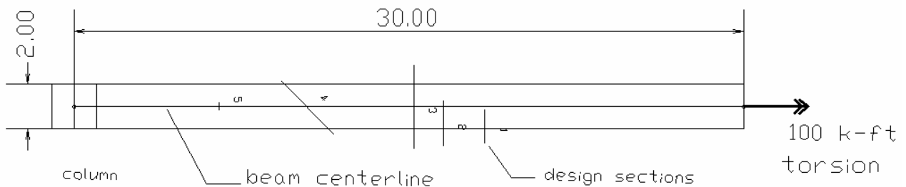
FIGURE 1 PLAN OF CANTILEVER BEAM SUBJECTED TO TORSION AT FREE END
